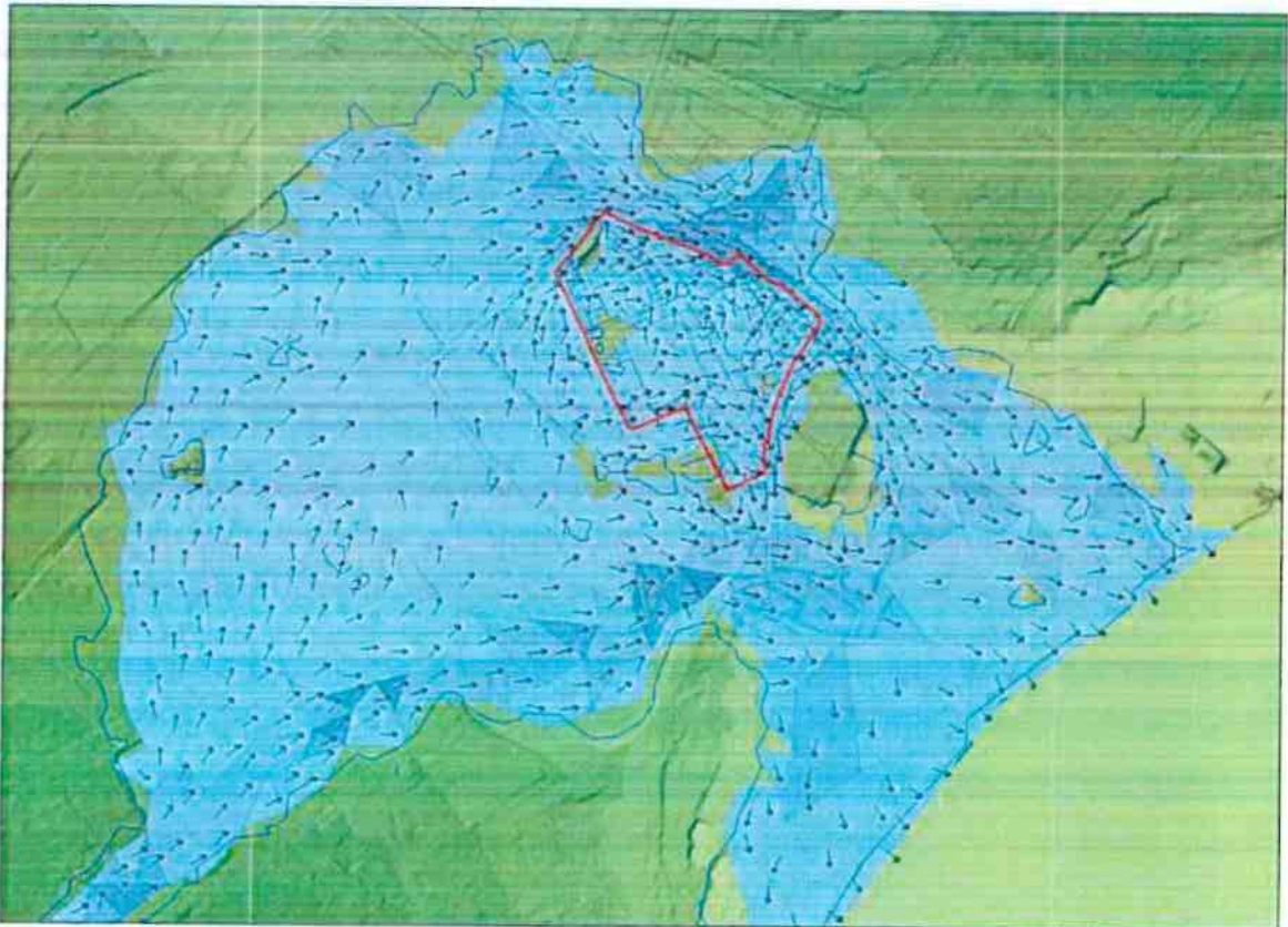
Plate 8.2: Maximum flood extent and depths resulting from a design flow with a peak of 500m 3 /s
